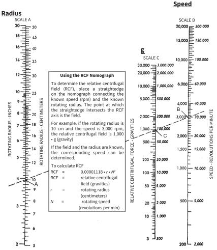
The distance measured from the rotor axis to the tip of the liquid inside the tubes at the greatest horizontal distance from the rotor axis is the rotating tip radius. The radius is listed for your convenience in the speed and force tables.
